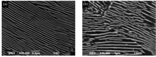
Fig.5. NLP82B inter-lamellar spacing of SEM samples (a) standard cooling, 74nm (b) slower cooling, 110nm.
