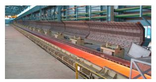
Fig.1. The Stelmor conveyor in the ROD2 Mill at CSC.
