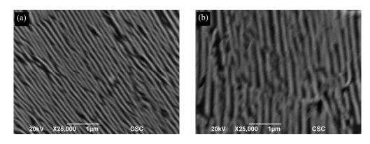
Fig.6. SWRH62A inter-lamellar spacing of SEM samples (a) standard cooling, 75nm (b) slower cooling, 105nm.
