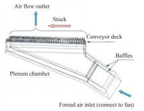
**Fig.2.** Assembly of a single plenum Stelmor air conveyor system.
